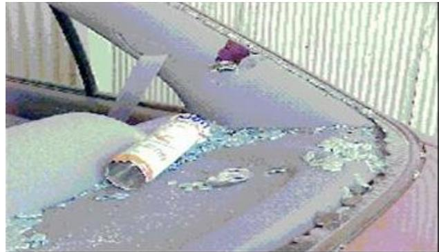
The incident pictured above happened at a refinery in Beaumont. A deodorant spray can was left in the back of the vehicle that was parked in an open space in the middle of a hot, sunny day.
