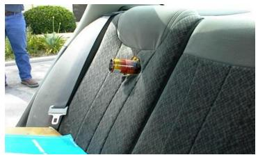
The pictures above are of a pressurized can that exploded in a person's vehicle and imbedded itself in the back seat of the car and through a back window. The temperature outside of the closed up vehicle was about 100 degrees F.
