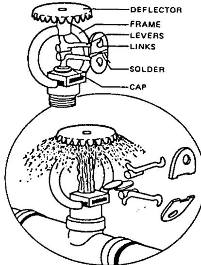
A typical fusible link type sprinkler head is shown in the picture below.
