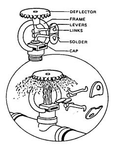
A typical fusible link type sprinkler head is shown in the picture below.
