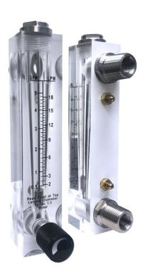
AdvanTech Aqua<sup>™</sup> Stainless Steel, Dual Scale Flow Meters are manufactured using an acrylic body with stainless steel internals, top cap, and fittings. AdvanTech Aqua<sup>™</sup> Flow Meters are individually calibrated using state of the art equipment, ensuring precise measurements.
