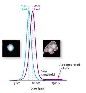
**PELLET AGGLOMERATION** is an inevitable property of the coating process. Obtained agglomerates are a common cause for process down time and directly affect the final product yield and coat integrity.
