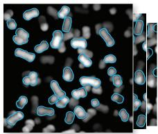
The objective of pelletisation is to produce spherical pellets with narrow size distribution and good abrasion resistance. **PATVIS** APA can be used to evaluate visually and numerically the **size and shape distribution of produced pellets**, which are key variables affecting the extrusion-spheronization process yield and quality.
