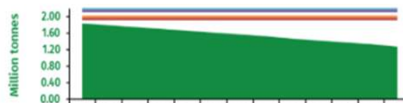
Municipal incineration capacity and available waste in the South West (with Northacre and Hill Barton)
