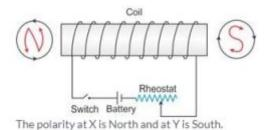
By increasing the number of turns of winding in the solenoid, the strength of the electromagnet can be increased.
