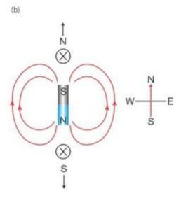
(c) Magnitude of magnetic field at neutral points is zero. It is so because at these points, the magnetic field of the magnet is equal in magnitude to the earth's horizontal magnetic field, but it is in opposite direction. Hence, they cancel each other.
