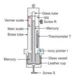
To measure the atmospheric pressure, first the leather cup is raised up or lowered down with the help of the screw S so that the ivory pointer I just touches the mercury level in the glass vessel. The position of the mercury level in the barometer tube is noted with the help of main scale and the vernier scale. The sum of the vernier scale reading to the main scale reading gives the barometric height.
