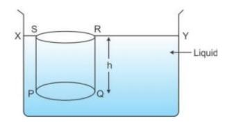
Total thrust exerted on the surface PQ
