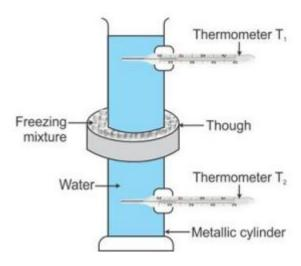
Hope's apparatus consists of a tall metallic cylinder provided with two side openings P and Q, P near the top and Q near the bottom, fitted with thermometers  $T_1$  and  $T_2$  in them. The central part of the cylinder is surrounded with a cylindrical trough containing a freezing mixture of ice and salt. The cylinder is fitted with pure water at room temperature.
