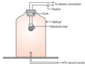
An electric bell is suspended inside an airtight glass bell jar. The bell jar is connected to a vacuum pump as shown in figure. As the circuit of electric bell is completed by pressing the key, the hammer of the electric bell begins to strike the gong repeatedly due to which sound is heard.
