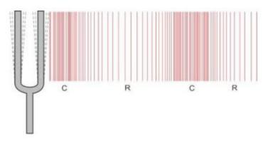
Compressions are the regions of high density where the particles of the medium come very close to each other and rarefactions are the regions of low density where the particles of the medium move away from each other.
