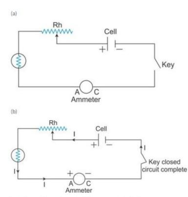
(c) A rheostat is used to control the current in the circuit.
