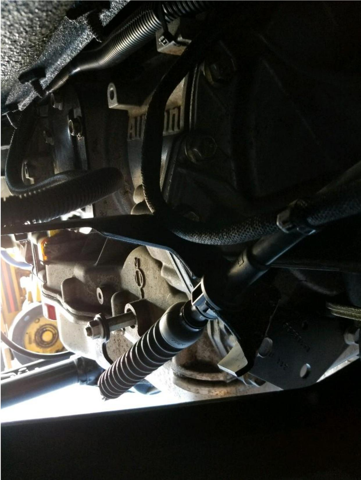
6. Now you will need to install the lower cable into the lower shift cable mounting bracket. You will hear it snap into position.
