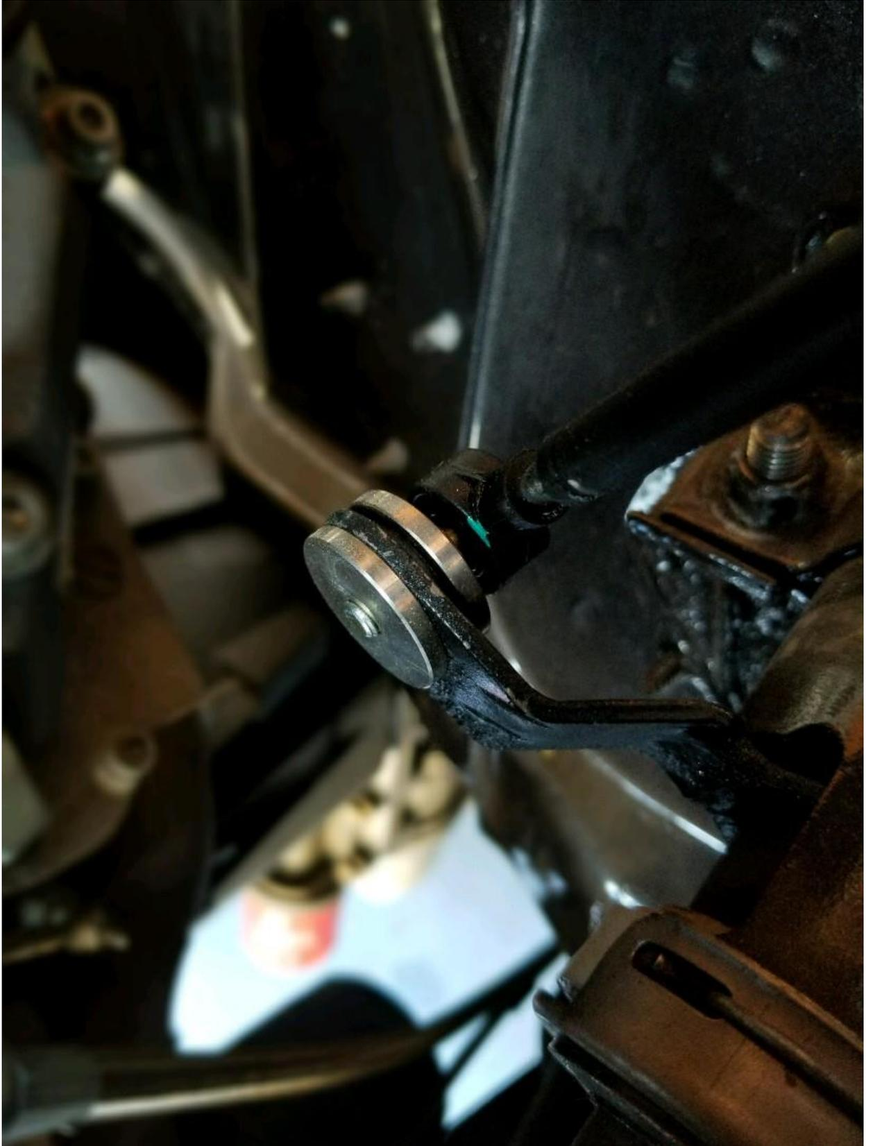
11. *Next you will snap the upper shift cable eyelet onto the 1/4" stud. Make sure it is seated in the groove.*
