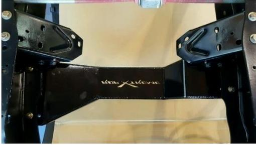
*10. Loosely install D/S & P/S lower engine mounts using the provided (6) six M10 x 1.5 x 30mm Flange Head Bolts and (6) M10 x 1.5mm Flange Head Lock Nuts.*
