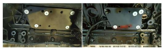
2. Install D/S upper engine mount bracket to engine mount plate and fasten using the provided (1) M10 x1.5 x 20mm Flange Head Bolt and (5) five M10 x1.5 x 25mm Flange Head Bolts. Torque using the provided Torque-Tension chart to determine proper bolt torque.
