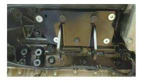
3. Install P/S upper engine mount bracket to engine mount plate and fasten using the provided (1) one M10 x1.5 x 20mm Flange Head Bolt and (2) two M10 x1.5 x 25mm Flange Head Bolts. Install the (1) one M10 x1.5 x 20mm Flange Head Bolt in the forward most hole. This placement is critical! If a 25mm long bolt is threaded into this hole it will come in contact and pinch
