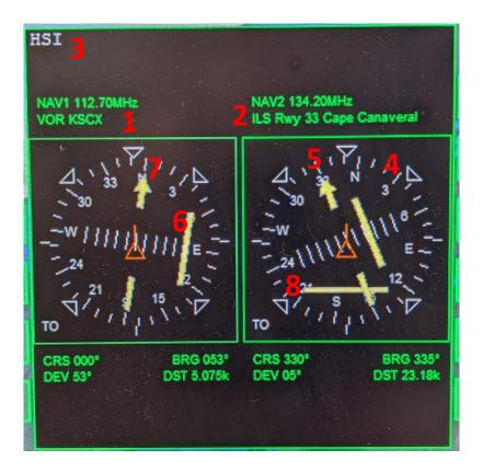
• NAV – The frequency at which the navigation indicator is broadcasting, it is specific to individual locations.(Kennedy Space Center- 112.70 MHz; Runway 33 at Cape Canaveral 134.20 MHz).In the orbiter, when programmed, the VOR for KSC will be received immediately. The ILS for Runway 33, when programmed, will be received 30 kilometers from the runway.
