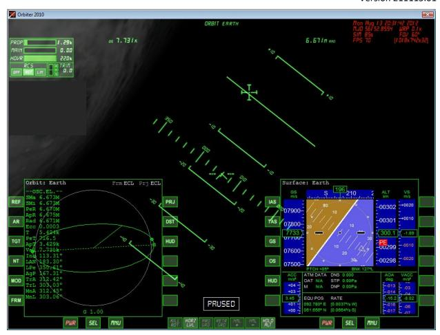
When the HUD is in "Orbit Earth" mode your flight path ladder is aligned with the orbital plane instead of the horizon plane, and there is a ribbon showing your orbital azimuth angle. It also shows indicators for pro-grade (the direction of your orbital velocity vector) and retrograde (the opposite direction). When in pro-grade your orbital plane is 000 degrees and the azimuth angle is 000 degrees, when in retrograde your orbital plane is 180 degrees and the azimuth angle is 00 degrees.
