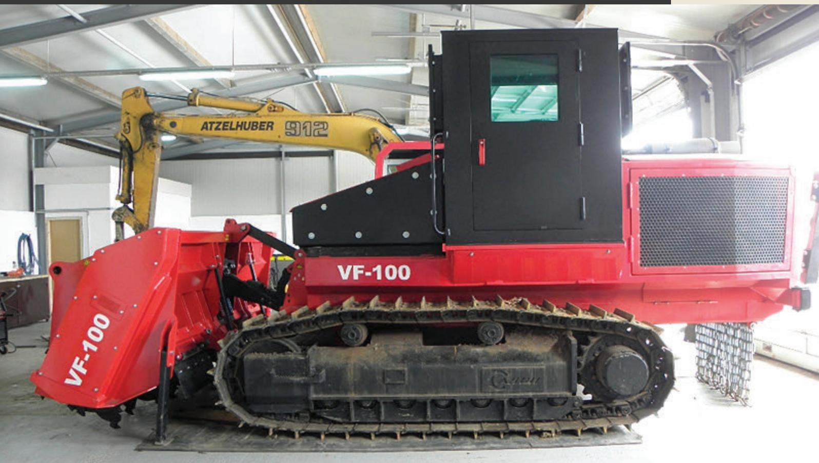
The VF-100, heavy demining machine, has been tested and certified by the Croatian Mine Action Center (CROMAC) Center for Testing and Research, and meets all requirements for use in humanitarian demining activities, passing tests on all anti-tank and anti-personnel mines
