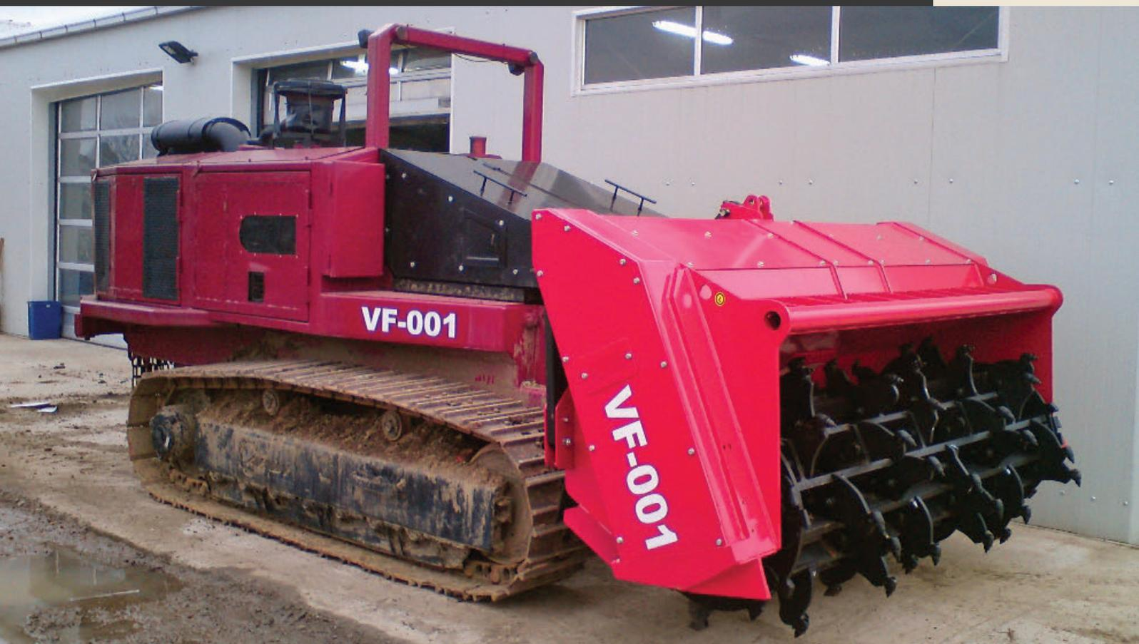
The VF-001, medium-sized demining machine, has been tested and certified by the Croatian Mine Action Center (CROMAC) Center for Testing and Research, and meets all requirements for use in humanitarian demining activities, passing tests on all anti-tank and anti-personnel mines.
