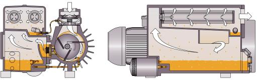
The machine works on the rotary vane principle.
