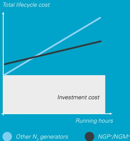
With an air factor of 1.8 (at 95%) to 5.5 (at 99.999%) and a special cycle time modulation algorithm, the running cost of the new NGP+ can be reduced by 50%, compared to other N<sub>2</sub> generators.
