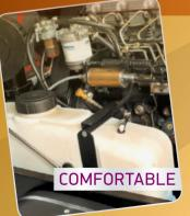
made of transparent plastic material for immediate level checking. Also fitted with a wide filler inlet.
