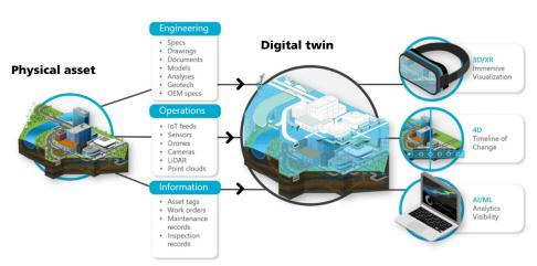
✓ Digital twins are continuously updated with data from the physical asset. This data is used to understand and model the asset's performance.
