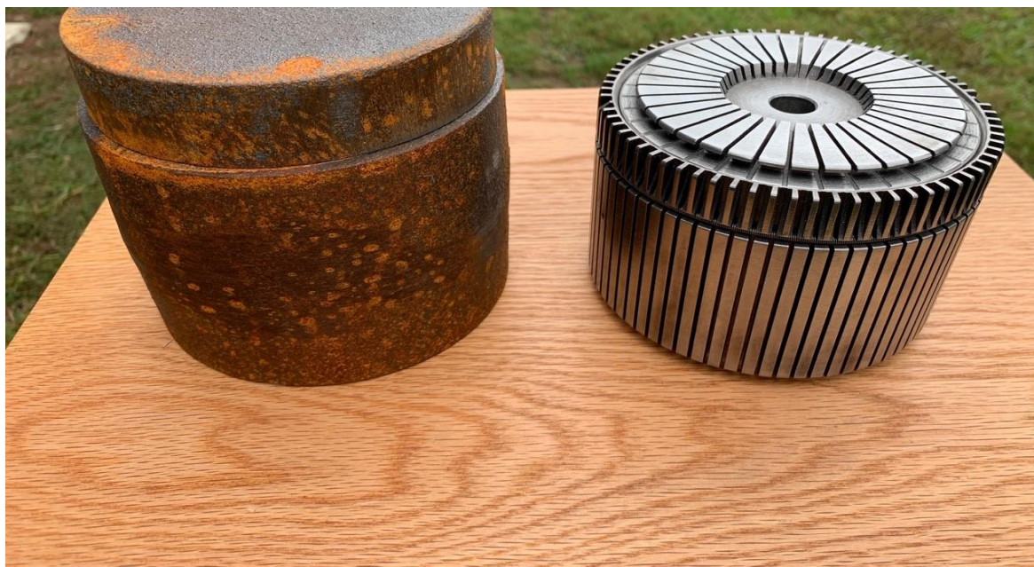
Left - Rough Cylinder and Ribber Dial Castings Right - Machined Cylinder and Ribber Dail
