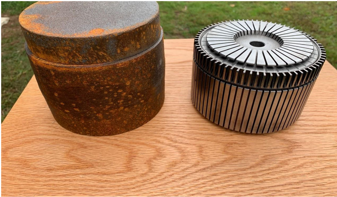
Left - Rough Cylinder and Ribber Dial Castings Right - Machined Cylinder and Ribber Dail
