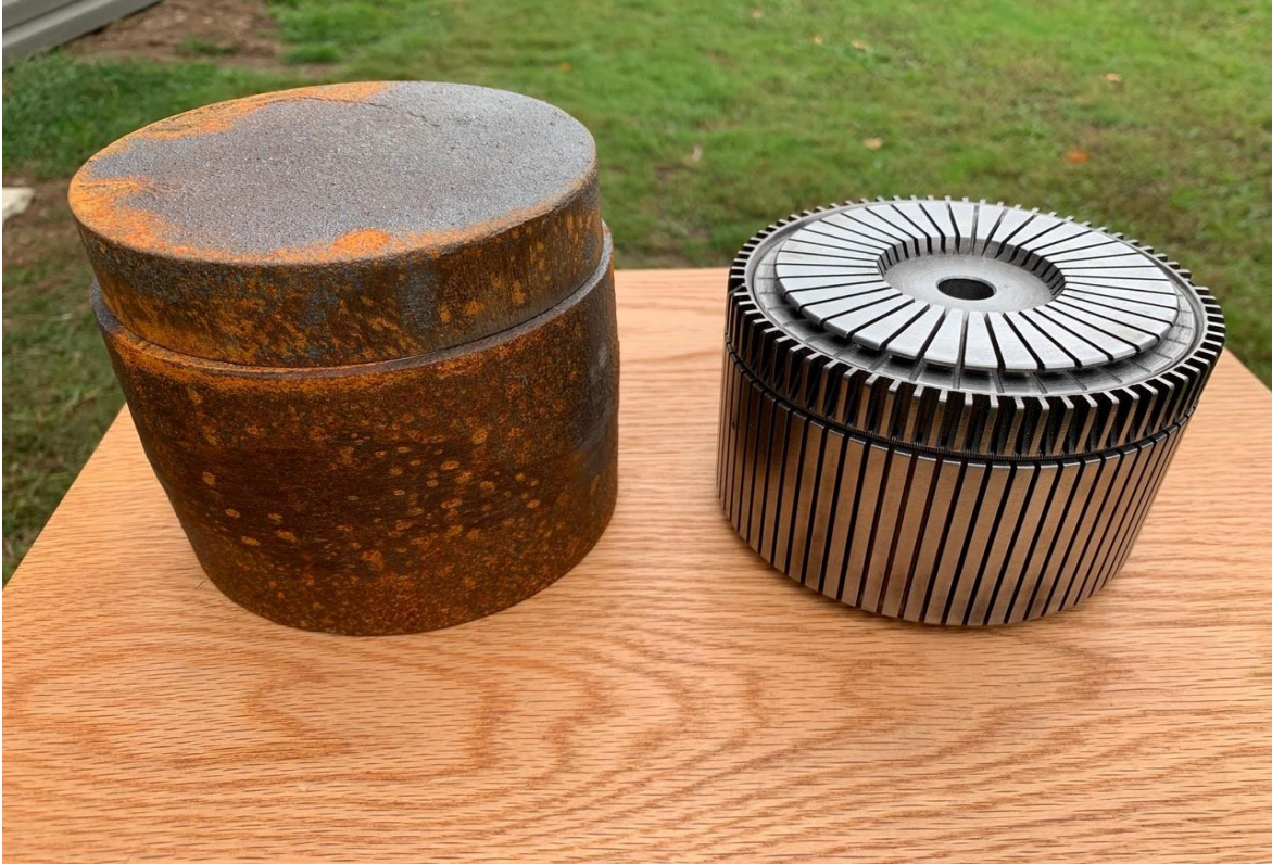
Left - Rough Cylinder and Ribber Dial Castings Right - Machined Cylinder and Ribber Dial
