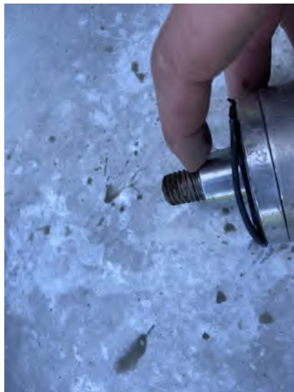
Photo 4: view of check-valve at top of sediment core sample barrel while cleaning
