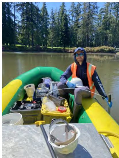
Photo 1: view of IP-C lakebed water sampling with peristaltic pump
