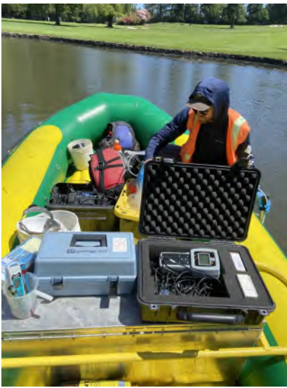
Photo 2: another view of IP-C lakebed water sampling with peristaltic pump.
