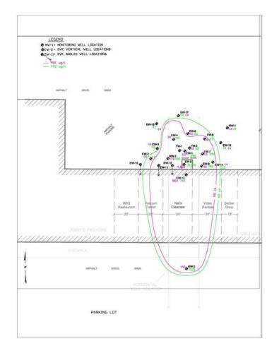
ERH electrodes were installed below grade inside the operating dry cleaning business and above grade outside the business in the adjacent parking lot. A total of 11 electrodes (co-located vapor recovery) and vapor recovery wells (3 located inside and 9 located outside) were used to heat the subsurface and remove the contaminants. Electrodes were installed at a depth of 8 to 28 feet bgs with a protective outer sleeve extending to the surface.
