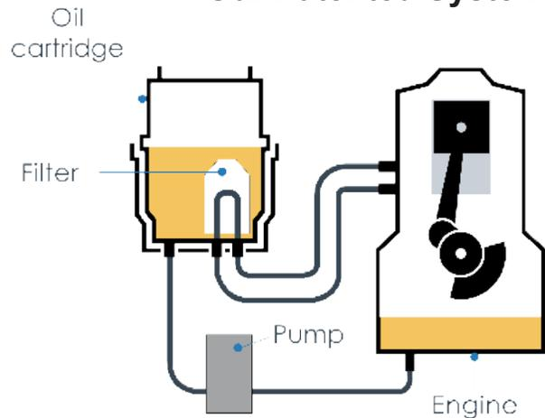
It is made up of a **removeable sealed oil cartridge** which contains the oil filter and tailored amount of oil as per the manufacturers recommendation. This connects to a fixed docking unit and oil is transferred to and from the engine sump using a keypad and pump control system.
