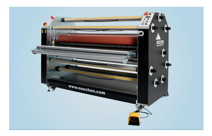
The Neschen HotLam 1650 DoubleH is a bi-directional laminator for efficient operation of all cold and hot applications. The high production speed, numerous unwind and rewind auto-grip shafts, pneumatically operated nip system, and integrated longitudinal cutting system guarantee high production output. The smart configuration of the four main rollers allows for a broad range of applications across mounting, laminating and encapsulating.
