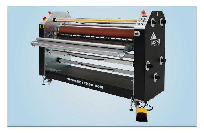
The Neschen HotLam 1650 TH is a real work horse. This powerful laminator combines efficiency and industrial performance with master-level results. Thanks to its sophisticated roller concept, pneumatically operated nip system, swing-out supply shafts, and roll-to-roll capabilities, the Neschen HotLam 1650 TH shows impressive results across wide-ranging applications. Designed to be operated by new or experienced users, this machine finds its place in every print finishing environment.
