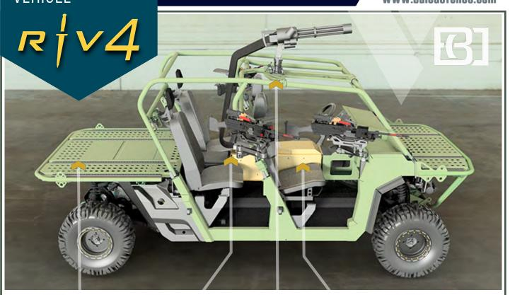
MODULAR MISSION KIT MOUNTING SYSTEM REMOVABLE M240/9 MG DUAL SWING ARM WEAPON MOUNT x3 QUICK DISCONNECT FOLDING ROPS WEAPON MOUNT CENTERALLY MOUNTED M134-D 3000 ROUND DAB3600 3-BAY AMMUNITION MAGAZINE
