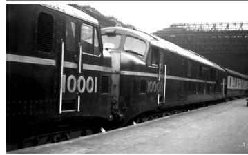
The Ivatt 'Twins', No's 10000 and 10001 were designed by H.G. Ivatt and built by the London, Midland and Scottish Railway (LMS) and English Electric (EE) at Derby Works in 1947/8. They were the first main line diesel locomotives and successfully set the shape of UK diesel traction for decades to come.
