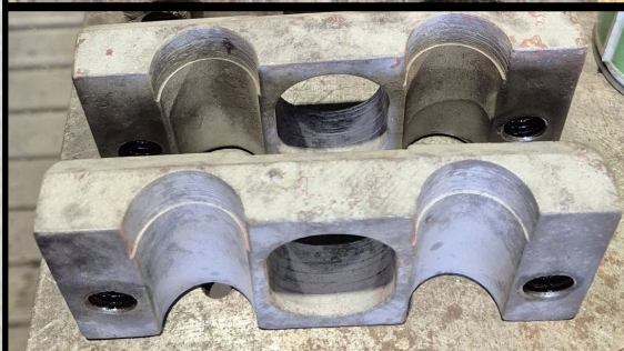
Above, Before and After. Parts cleaned in the sand - blaster box. Mark Langley
