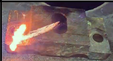
Left, the laser used to remove rust and dirt. Mark Langley.
