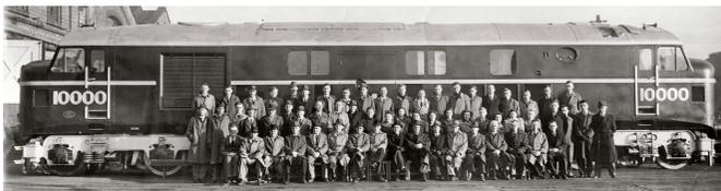
10000 was Britain's first mainline diesel locomotive. It was also the first British Co-Co locomotive in traffic. Co-Co is the notation used by railways for a locomotive with two bogies, each with three axles powered by electric transmission.
