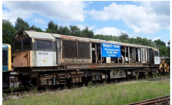
Utilising the proven class 58 chassis also increases the stability of the loco over the original design. The higher level of the 58 chassis compared to the original means that the crankshaft height of the 16SVT power unit will be lower to the rail height, as the engine will sit between the chassis longitudinal beams rather than above them, as in Ivatt's original design.
