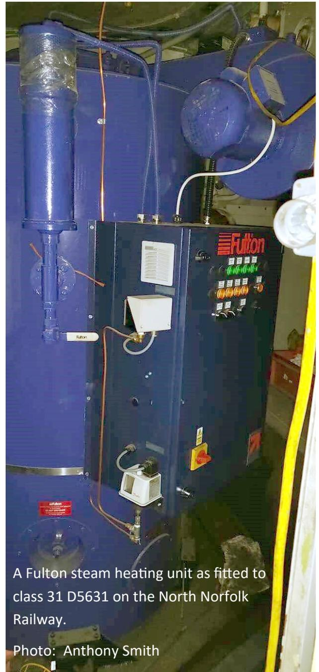
A Fulton steam heating unit as fitted to class 31 D5631 on the North Norfolk Railway.
