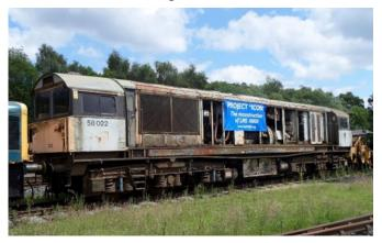
Utilising the proven class 58 chassis also increases the stability of the loco over the original design. The higher level of the 58 chassis compared to the original means that the crankshaft height of the 16SVT power unit will be lower to the rail height, as the engine will sit between the chassis longitudinal beams rather than above them, as in Ivatt's original design.
