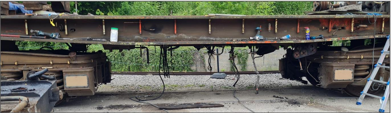
**Fuel tank removal, including draining fuel.**
