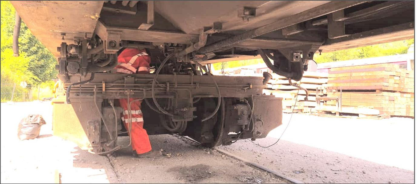
**Above:** A lot of work went unseen, underneath the chassis. Here we see a volunteer engrossed in work to separate the chassis from the bogies. Once the fuel tank was removed there was a lot of space, but not so amid the bogies!
