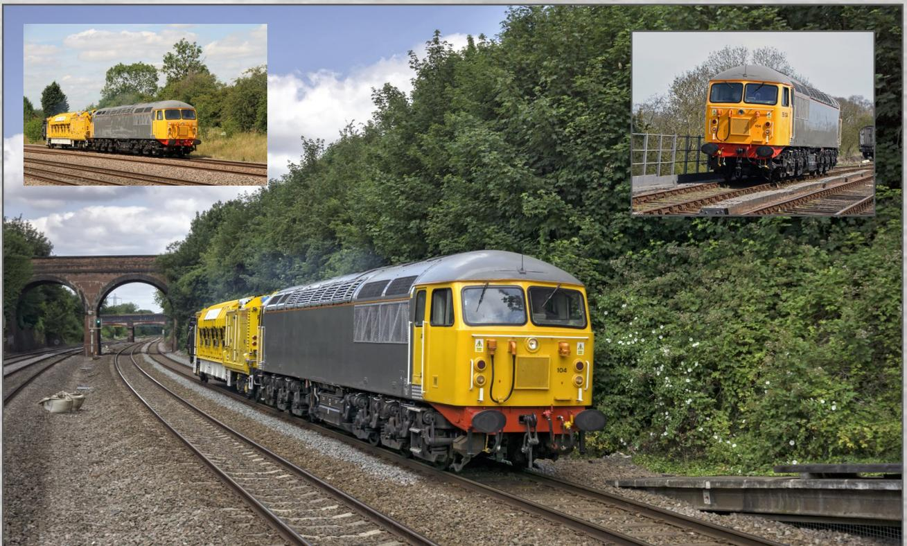
Such a rush of opportunities to obtain equipment has depleted our bank account just as much as it has filled Centenary Works! The main items remaining on our shopping list are class 37 braking gear and EM2 parts. We will have to strengthen the bogie suspension to take the additional weight carried in a diesel loco. Then there is wiring and bodywork. Plenty to keep us busy!
