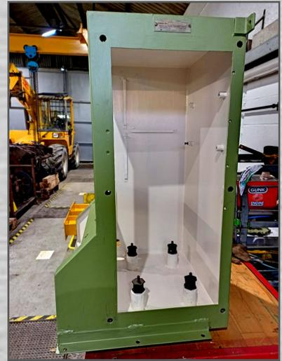
The apparatus inside the cubical has to be methodically documented, disconnected leaving the termination wiring behind. We also have to remove all termination blocks and overhaul them with new zinc plated bolts. The work area at the rear of the workshop is being reorganised to facilitate this activity, including reinforced plating over the inspection pit.
