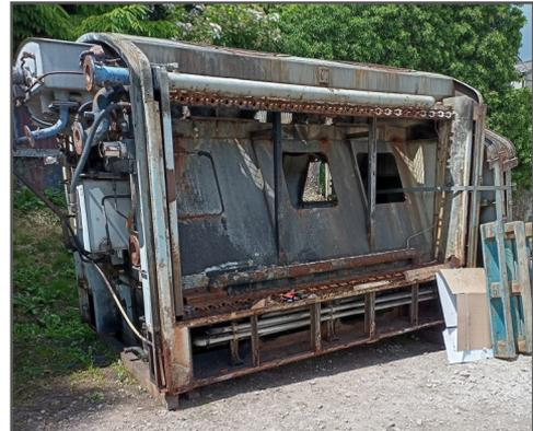
It will be cut to size suitable for the new loco. Meanwhile the cabs were removed and one is displayed at our visitor area.
