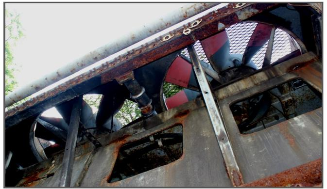
The cooling group was transported up to Centenary Works where it was cleaned.
