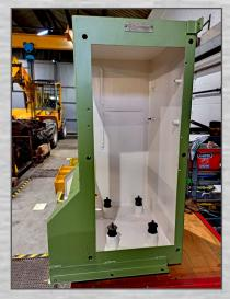
The apparatus inside the cubical has to be methodically documented, disconnected leaving the termination wiring behind. We also have to remove all termination blocks and overhaul them
