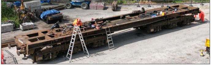
**Before and After!** Above: A drone photo of the chassis of 58022 showing work in progress to prepare it for the big event. Bob Hodgson, EVR. **Below:** After being lifted from the bogies, the chassis is seen on the ground before being turned over.
