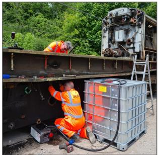
Fuel tank removal, including draining fuel.
