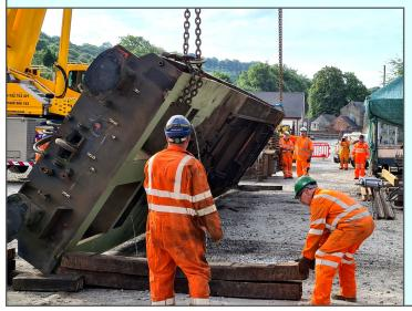
In this issue we focus on the 'Big Lift', the much awaited inversion of the loco chassis so we can work on its under side in preparation for matching it to the bogies.
