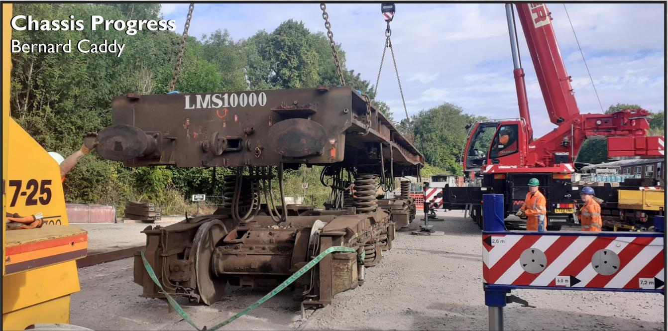
After the work of the previous eighteen months to strip it, our chassis was lifted off the bogies last summer, inverted, placed onto our Sturgeon wagon and sheeted over. Photos on this page show that process.
