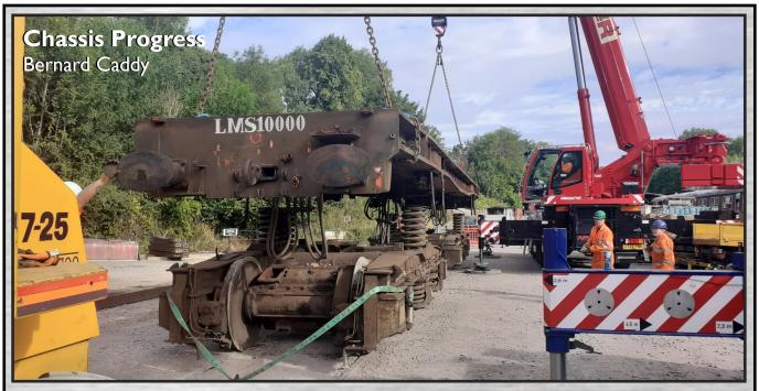
After the work of the previous eighteen months to strip it, our chassis was lifted off the bogies last summer, inverted, placed onto our Sturgeon wagon and sheeted over. Photos on this page show that process.
