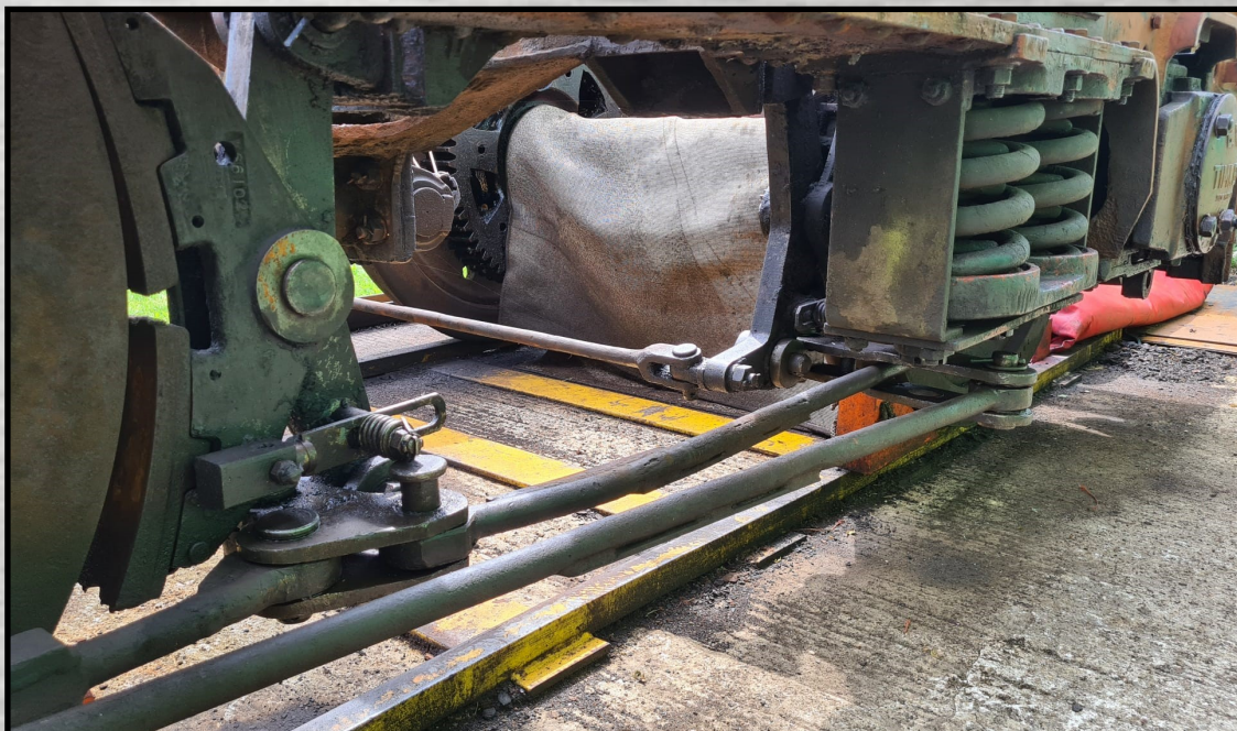
Bottom: With the leaf springs and the spring supports removed, a large space was revealed.
