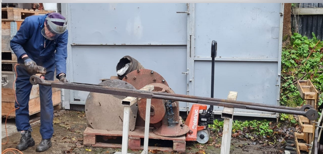
The rods of the brake system being cleaned and painted. Mark Langley
