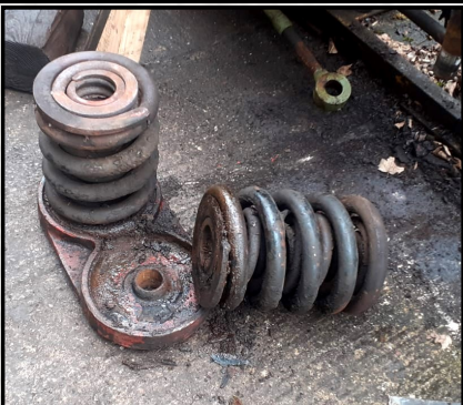
Above: This is the only way these pivot pins can be removed, there is no access from behind.
