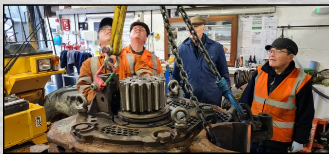
Lifting a traction motor. Mark Langley
