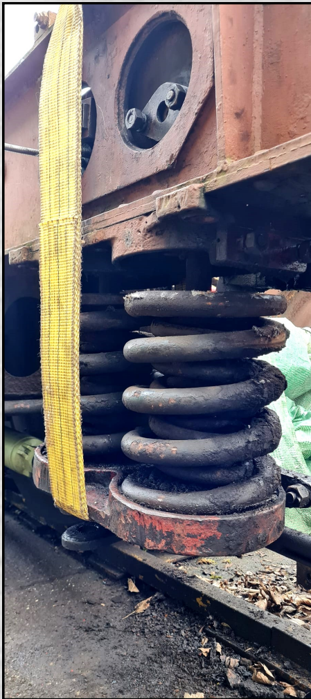
The process of lowering triple-nested coil springs from the bogie frame. Mark Langley
