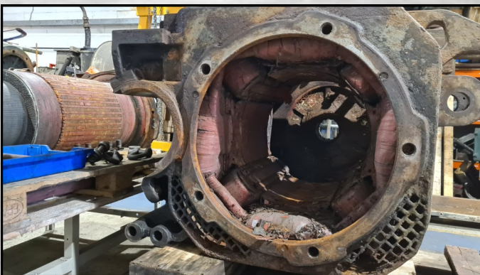
The inside of a traction motor! Bernard Caddy
