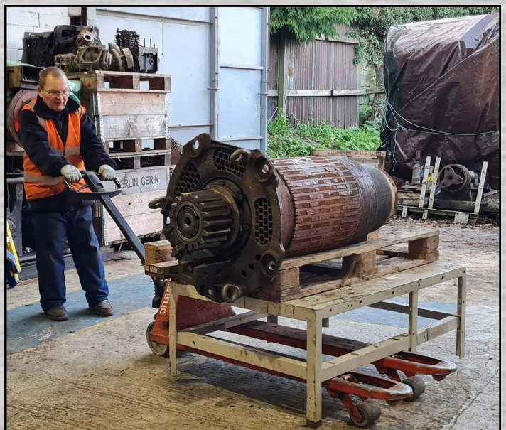
The traction motor's armature being positioned. Mark Langley
