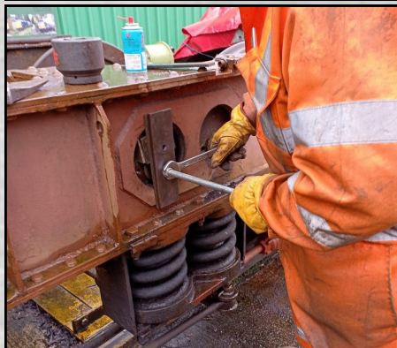
Above: This is the only way these pivot pins can be removed, there is no access from behind.
