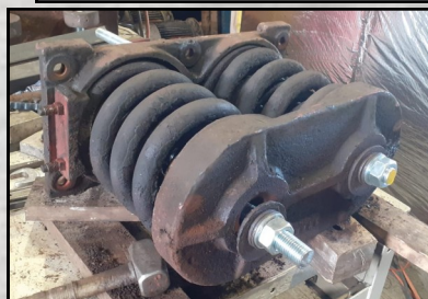
Above: This is the only way these pivot pins can be removed, there is no access from behind.
