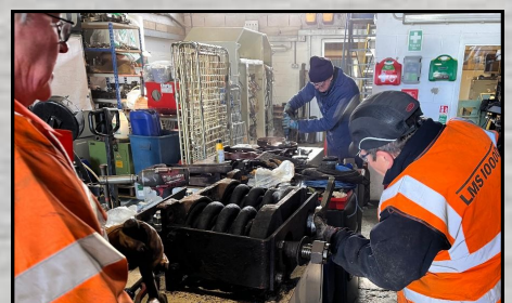
The coil springs were moved indoors to be cleaned. Anthony Pilkington
