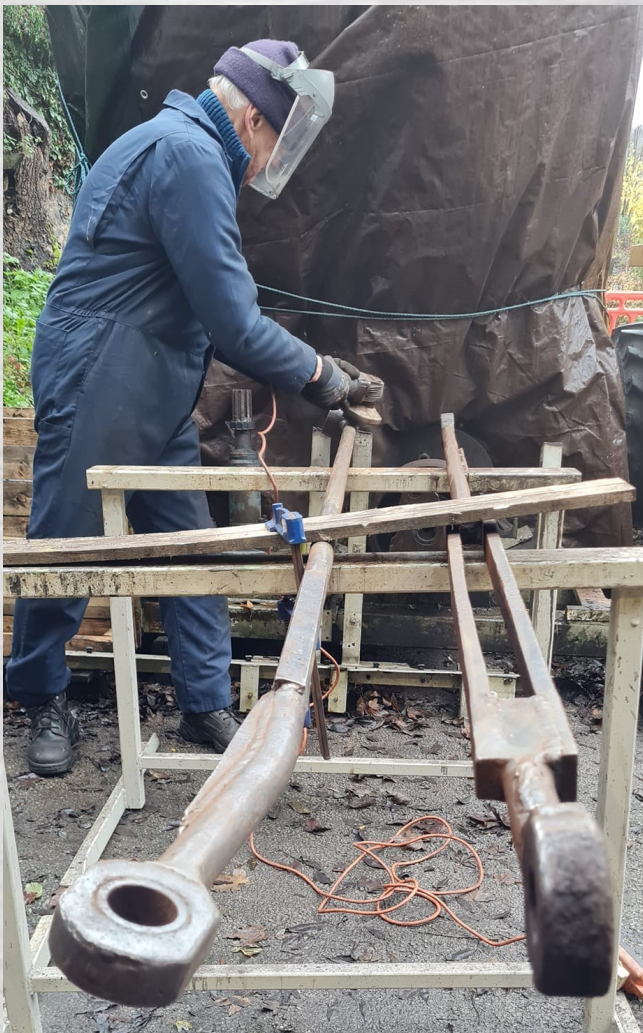
The rods of the brake system being cleaned and painted. Mark Langley
