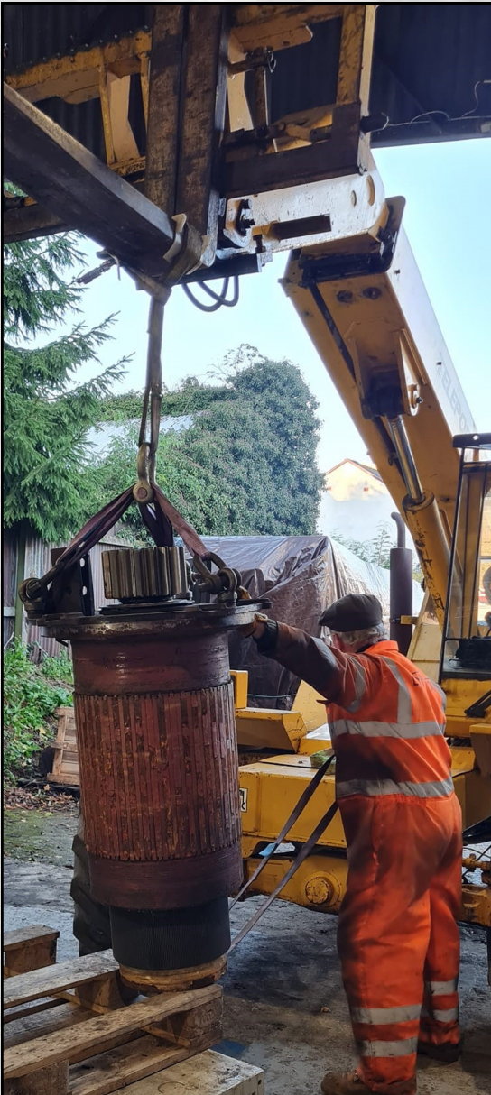
The traction motor's armature being lifted by the Telehandler. Mark Langley
