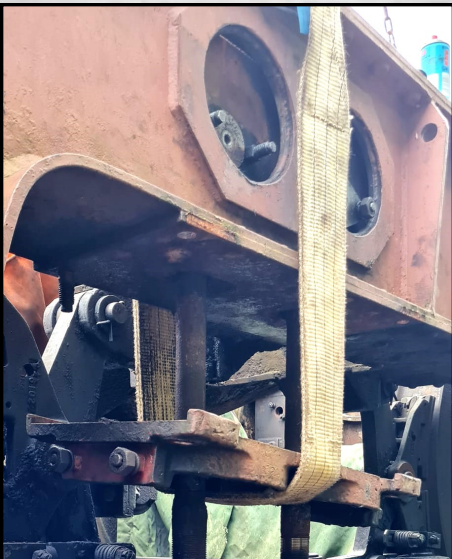
The process of lowering triple-nested coil springs from the bogie frame. Mark Langley
