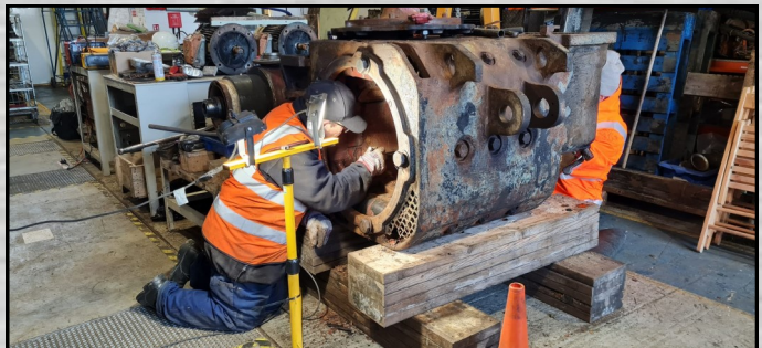
Inspecting a traction motor after removal of the armature. Mark Langley
