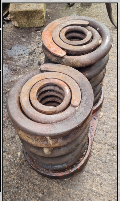
The process of lowering triple-nested coil springs from the bogie frame. Mark Langley
