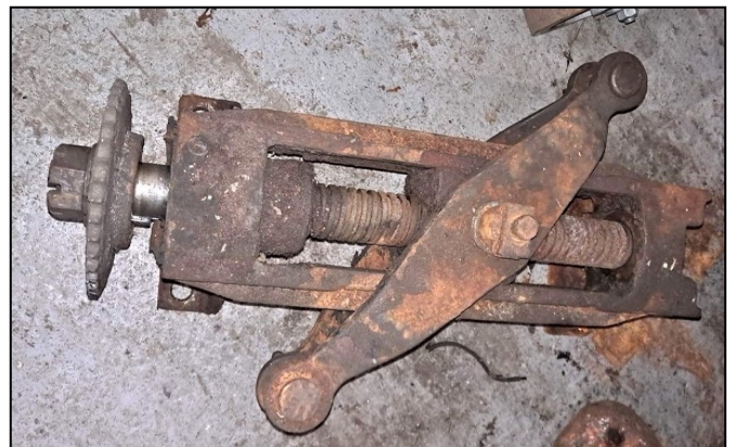
One of the handbrake mechanisms, chain driven from the handbrake wheel in the cab.
