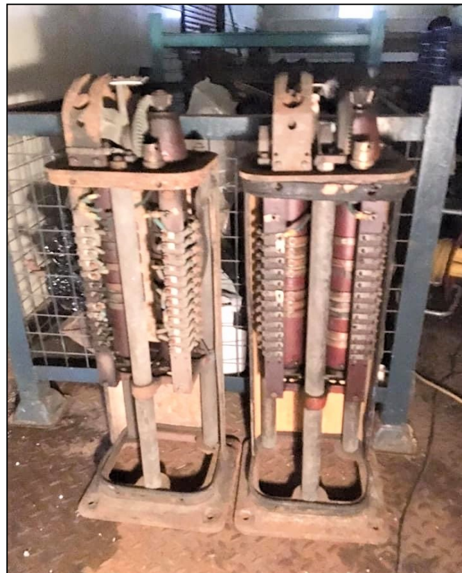
Two very rare items - control pedestals from a class 31/0 locomotive, These will be refurbished and modified for reuse on 10000. The mechanisms on the top will be removed and replaced with items identical to those on 10000/1.
