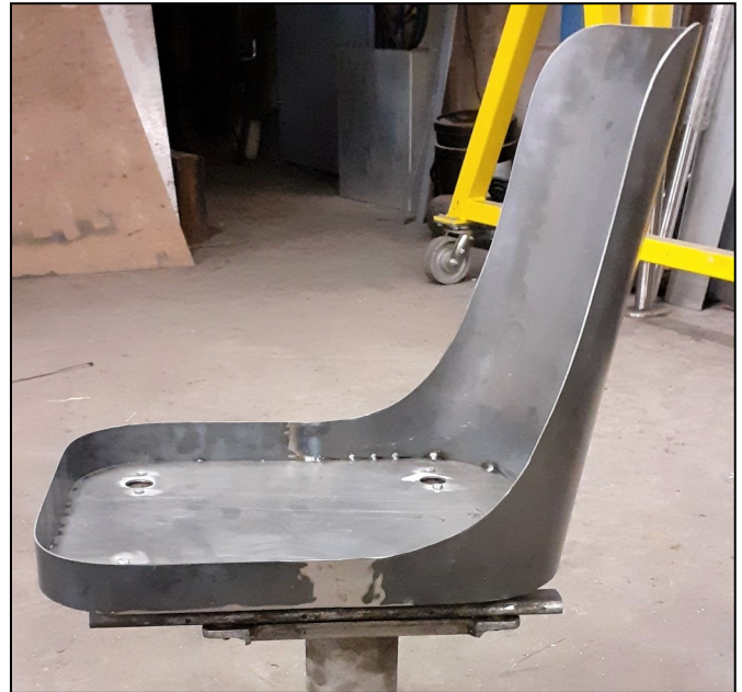
This version of the seat is a mock-up to check that all the angles and dimensions are correct before remanufacturing in thicker steel sheet.
