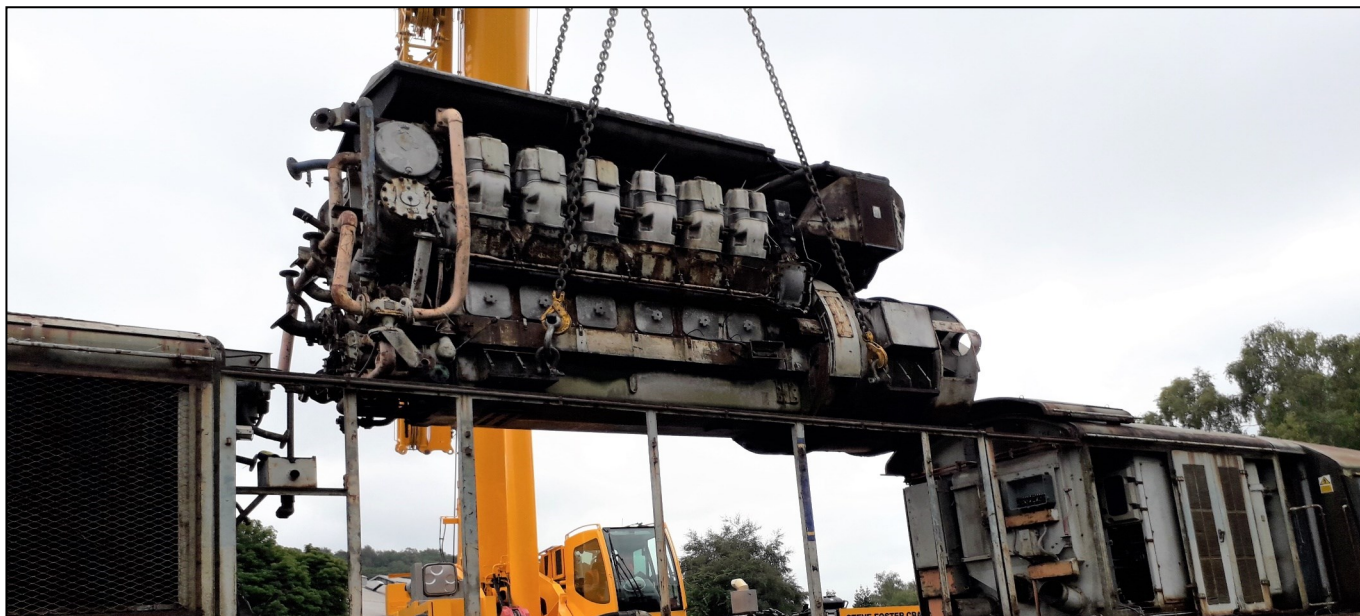
After some last minute difficulty with a stubborn engine mount, the power unit is finally free of the loco.
