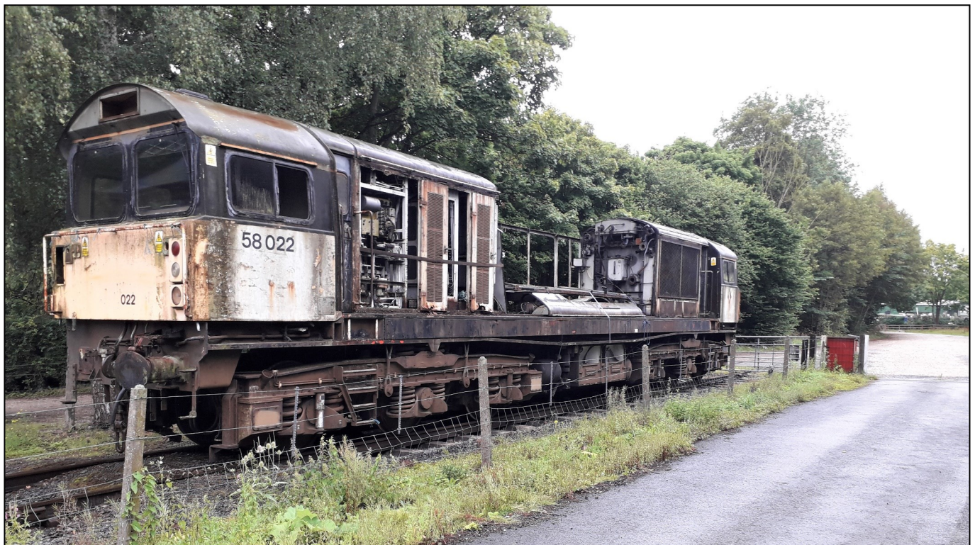
58022, minus its power unit, awaiting the arrival of the Allelys trailer.
