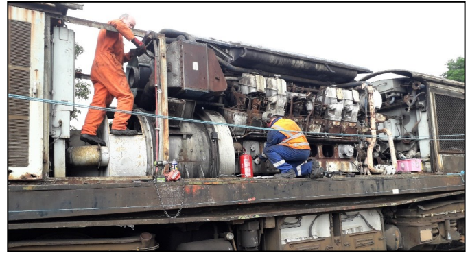
Bernard and Paul preparing the engine for removal.
