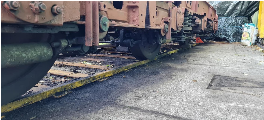
On the 16th Mark L spend a couple of hours scraping, chiselling and brushing off years worth of congealed brake muck from the bogies and bagging what could be reached underneath.
