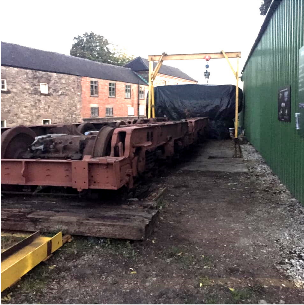
On the 16th Mark L spend a couple of hours scraping, chiselling and brushing off years worth of congealed brake muck from the bogies and bagging what could be reached underneath.
