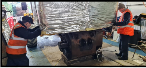
These photos show the oven frame being lowered over the traction motor. Photos: Mark Langley.
