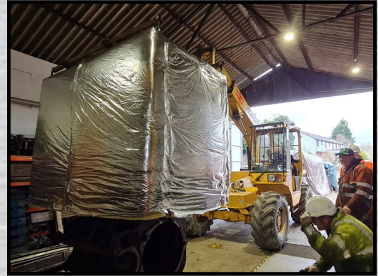
These photos show the oven frame being lowered over the traction motor. Photos: Mark Langley.
