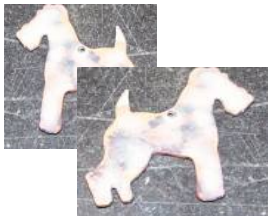
#6 Clean with Alcohol Flip piece. Coat back Side with Scalex to help reduce oxidization.
