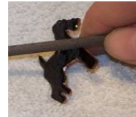
#23 File sharp edges from enamel Build up and burrs.
