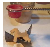
#14 Place on stand, add base coat (Top enamel).
