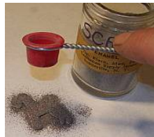
#7 Use counter enamel on opposite side of Scalex to coat back of piece.
