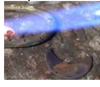
#5c Heat the finding till the silver solder melts.
