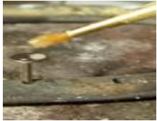
#5a Flux the piece and tack or other finding(s).
