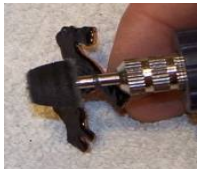
#24 Buff edges with Rotary tool to a Smooth surface.
