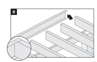
**Installing Rim Plate and Joist Blocking** (Drop Beam Scenario Only)
