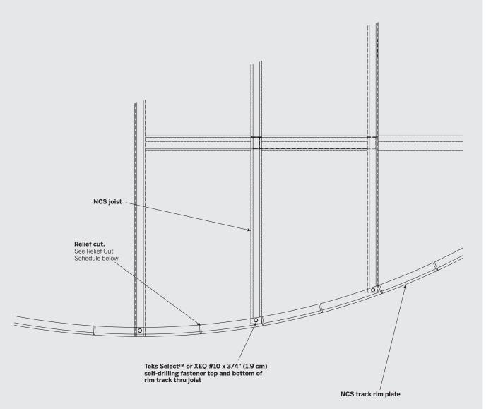
**RELIEF CUT SCHEDULE** NEW CASTLE STEEL TRACK TOP AND BOTTOM FLANGE RADIUS RADIUS 3' - 0" to 5' - 11" (91.4 cm to 180.3 cm) 2" (5.1 cm) 5' - 11" to 8' - 11" (180.3 cm to 271.8 cm) 4" (10.2 cm) 8' - 11" to 11' - 11" (271.8 cm to 363.2 cm) 6" (15.2 cm) 11' - 11" to 14' - 11" (363.2 cm to 454.0 cm) 8" (20.3 cm) 14' - 11" and above (454.0 cm and above) 10" (25.4 cm)
