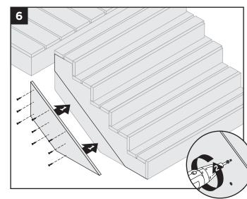
6. Fasten second fascia board (two 1x8 fascia boards are needed in most cases, as one fascia board will not cover stringers) to stair framing by screwing recommended decking with metal fasteners into the stair framing. Number of screws used would depend on width of fascia, if full 1x8 is used, three screws would be required. See Required Fasteners chart on page 6, column B.
