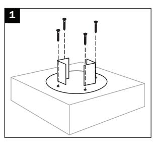
2. Install post cut to desired length, over post base.
