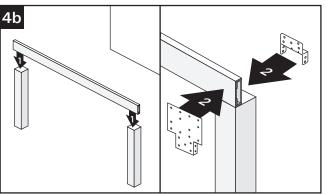
4b. Attach beam to post using NCS front beam bracket with required fasteners. See Required Fasteners chart on page 6, column A, for approved metal-to-metal fasteners for attaching brackets to beam.
