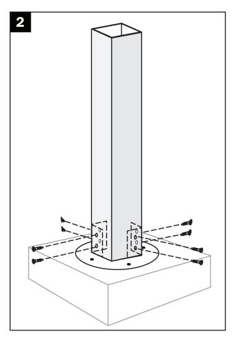
2A. Pre-drill 2 holes each side through post and post base with a 3/16" drill bit. Holes should be placed center line of post. 1 1/2" and 5" from base.
