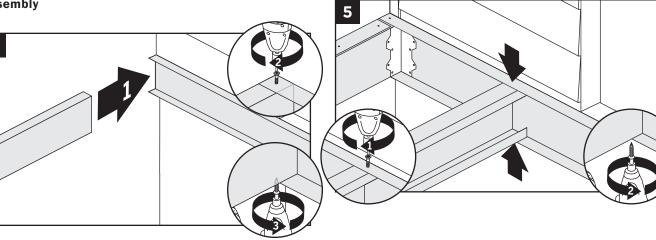
1a. Slide the joist within the flanges of the track and rest the outer end on the support post or beam. Fasten joist to track using required fasteners. See Required Fasteners chart on page 6, column A. Fasten through the track flange into the joist on top and bottom.
