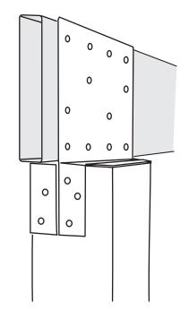
5. Secure cap with exterior grade metal adhesive and/or #10 x 3/4" (1.9 cm) self-tapping screws.
