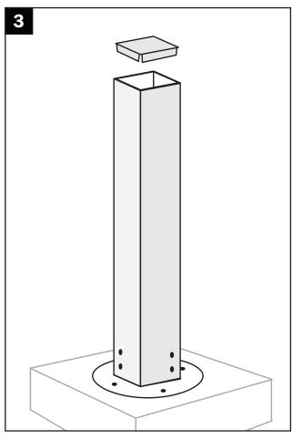
3. Secure post cap with exterior grade sealant.
