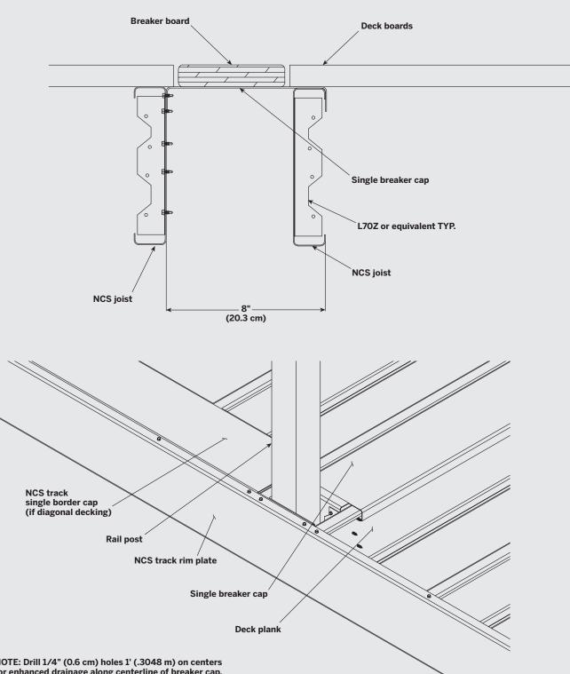
NOTE: Drill 1/4" (0.6 cm) holes 1' (.3048 m) on centers for enhanced drainage along centerline of breaker cap.
