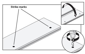
2. Flip board over so that bottom of board faces up and shows strike marks from the screws. Using a paddle drill bit, carefully drill holes to the depth of the fastener heads in the joist. Flip board over so that drilled holes
