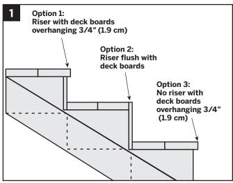
Install the deck boards as required by local code. Check with your local building code inspector for requirements.
