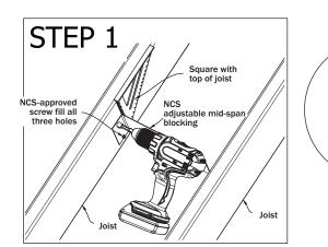
Place single flange block against joist a minimum of 1/4" above joist flange return. Plumb, fill all three holes with NCS-approved screws.
