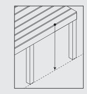
To determine the appropriate riser height, measure from the top of the deck surface to the landing.
