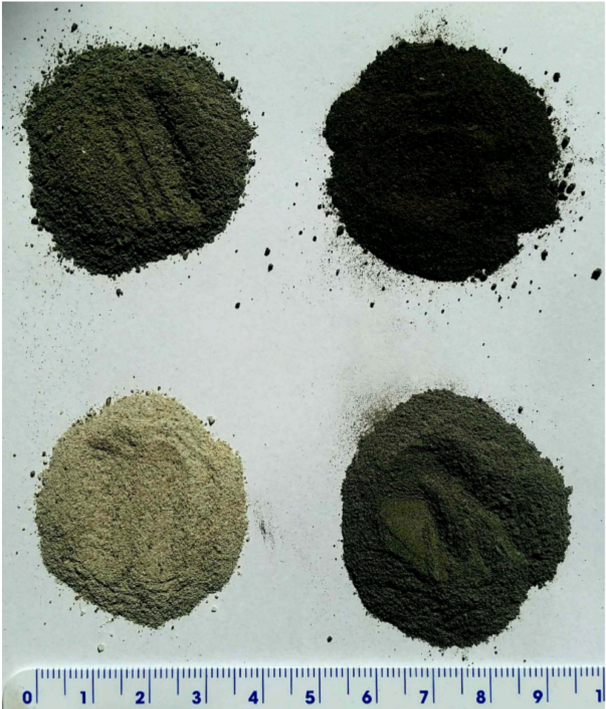
Image 4: Photo of four types of lunar regolith: EAC-1 (top left), JSC-2A (top right), LHT3M (bottom left), and FJS-1 (bottom right). The scale bar is in cm. Source: https://link.springer.com/article/10.1007/s10853-018-3101-y
