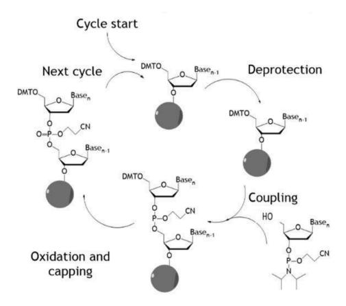
Traditional oligonucleotide synthesis, Source: Manufacturing Chemist
