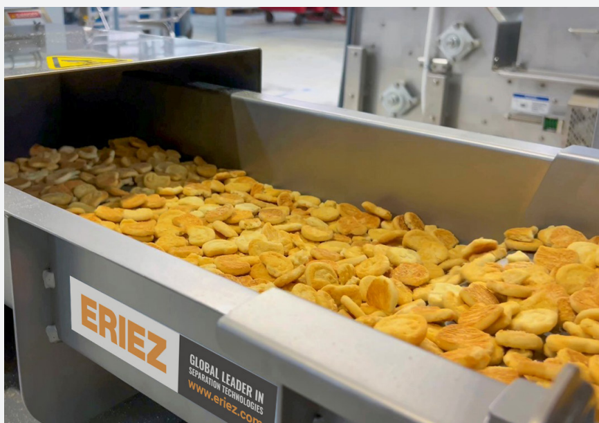
An Eriez Vibratory Feeder metering out product into the X-ray Inspection System
