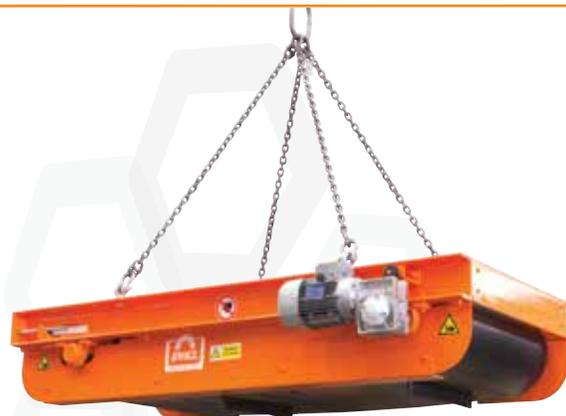
Suspended Magnetic Separators are designed for applications where ferrous contaminants are to be removed from bulk products – either on a moving conveyor belt or chute.
